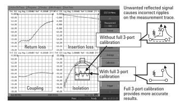
Figure 12. Full 3-port calibration in coupler measurement
