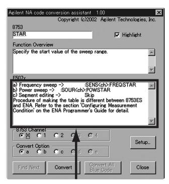
Figure 33. Quick Help shows equivalent GPIB commands and code conversion tips
