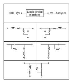
Figure 21. Pre-defined models of matching circuit embedding
