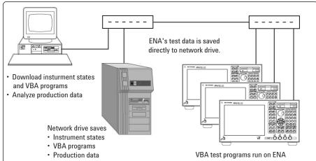
Figure 9. ENA factory automation example
