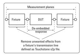
Figure 18. De-embedding for removing fixture effects
