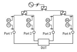
Figure 22. 4-port ENA hardware architecture
