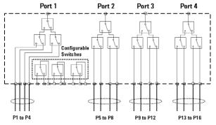
Figure 25-2. E5091A-016 16-port configuration block diagram
