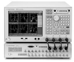
Figure 24. ENA and E5091A-016 test set
