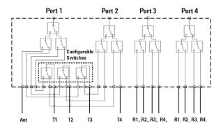
Figure 25-1. E5091A-016 13-port configuration block diagram
