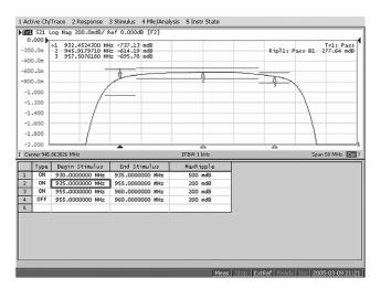
Figure 11. Ripple limit test
