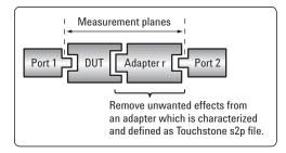
Figure 19. De-embedding for mixed-connector device measurements
