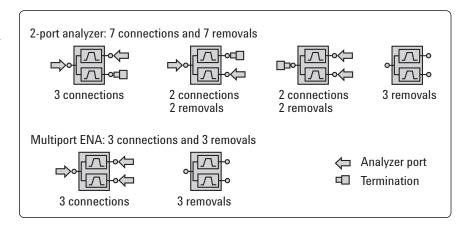
Figure 23. Number of connections/removals needed for duplexer test
