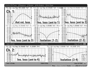
Figure 29. 4-way power divider measurement example using two full 4-port calibrations
