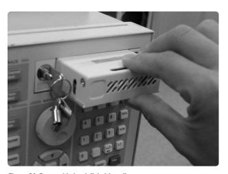
Figure 34. Removable hard disk drive allows you to secure and protect your confidential data
