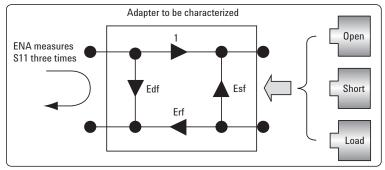
Figure 14. Adapter characterization (single directional method)
